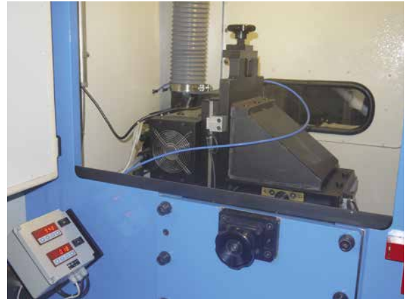
Combined system for adjusting the position of the electric head
