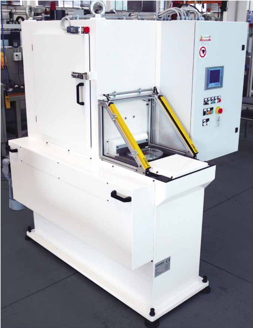
Combined system for setting of the electric grinding head position
