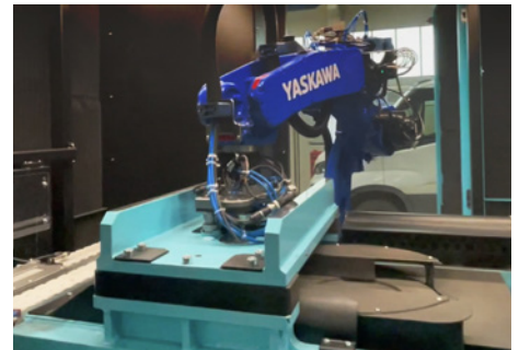
Smoothing of the pad surface
